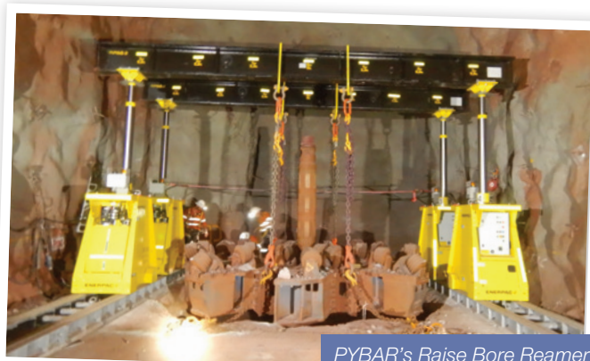
PYBAR’s Raise Bore Reamer Lifting Gantry system.
